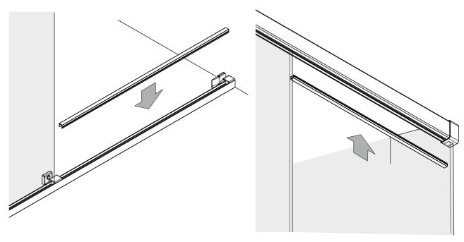
Cut a section of the aluminium Infill profile to fit the Underframe between the Floor Guide and the Shoe assembly. Clip into position.
