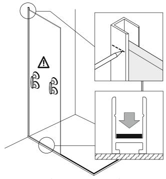
Lay strips of rubber inside the underframe to cushion the in-line and return glass panels. Using glass lifters, first place the in-line panel in position.
