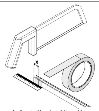
Cut dimension X from the straight end of the underframe - not the mitred end.
