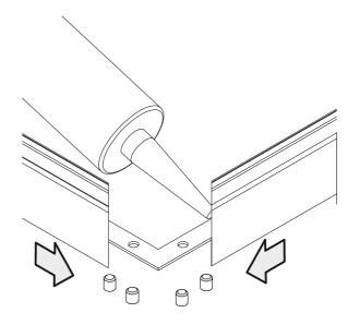
Apply silicone to the mitre of the underframe and assemble using the right angle connector.
