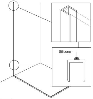
Remove both Surface Profiles and cut them to length so that they will be level with the top of their respective glass panels.
