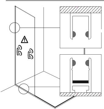
Apply a bead of silicone to both inside faces of the underframe and the 17mm Surface Profile as shown and lift the In-line glass panel back into position. Similarly, apply a bead of silicone to the return section of the underframe and to the 24mm Surface Profile and fit the Return glass
