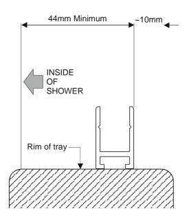
If a shower tray is used, ensure that there is at least 44mm of flat rim behind the front edge of the underframe to leave space for the floor guide. Ideally, both sections of the underframe should be about 10mm back from the outside edge of the tray.
