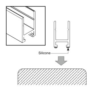
Apply beads of silicone to the bottom of the underframe as shown and apply a small amount to each end where the underframe will sit against the wall.
