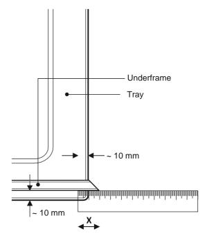
Place the front section of underframe in position on the rim of the tray and mark the position of its front edge.
