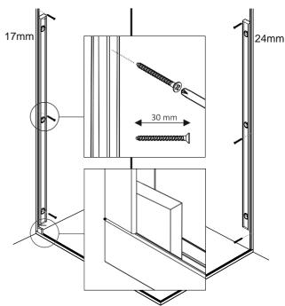
Place the 17mm Surface Profile in position at the in-line panel end of the underframe and the 24mm Surface Profile at the return panel end using the 10mm Spacer to ensure alignment. Use a long spirit level to ensure that they are vertical. Mark the screw hole positions. Drill the wall, fit the wall plugs and screw the Profiles in place.
