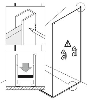
Remove the inline panel and then place the return glass panel in position.
