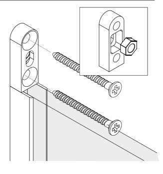
Place the M6 nut in the recess in the back of the wall plate using a smear of silicone to hold it in position at the top of the recess during assembly.
