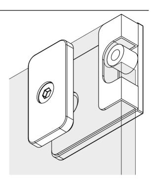
Assemble the plates of the return bracket assembly to the top corner of the return panel as shown above, ensuring that the transparent gaskets are on both sides of the glass and that the top edge of the plates is level with the top edge of the glass.
