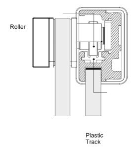
Lift the door into position on the Rail. In smaller enclosures, you may need to lower the bottom of the door into the Floor Guide before lifting it and locating the rollers on the plastic track. Check that the door is correctly located and can run smoothly
