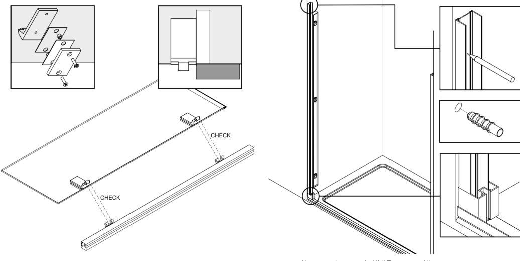
Lay the glass Door horizontally on cushioned trestles or similar and assemble the hinges to the glass Door as shown. Ensure that the clear plastic sleeves are fitted inside the holes in the glass and that gaskets are placed either side of the glass.
