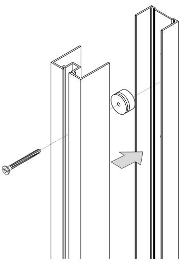
Assemble the inner wall frames to the outer frames using the longer screws provided in the remaining holes.
