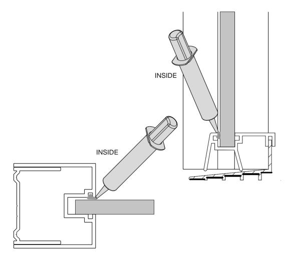
Seal around the glass panel on the inside of the shower only as shown above. Push or peg the glass away from you so that you have sufficient space between the glass and the frame and apply a thin bead of silicone.
