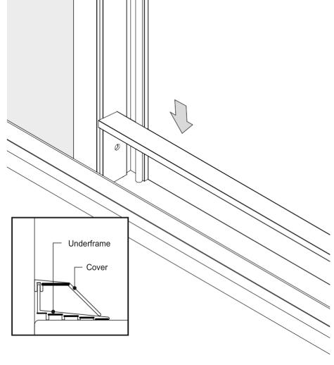
Position the Centre Frame assemblies and lower the Top Frame assembly in to position.
