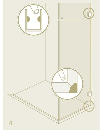
Fit the inner part of the glass-to-glass bracket to the glass return panel, so the clear plastic gasket is aligned with the edge of the glass. Attach the faceplate through the hole in
