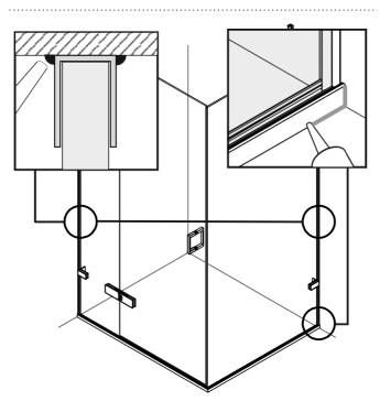
Run a small bead of silicone along the outside edge of the underframe where it meets the tray or floor and on the vertical edges where it meets the wall.
