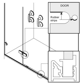
Insert two short pieces of self adhesive rubber strip in each door hinge slot as shown.
