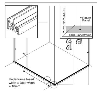
Using suction glass lifters, lift the In Line and Return panels into their respective wall profiles and carefully lower into the underframe channel. Ensure that the Return panel is pulled forward in the underframe to align as shown.
