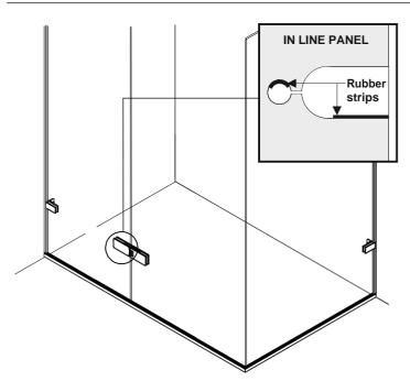
Insert two short pieces of self adhesive rubber strip into each In Line panel hinge slot as shown. Disassemble the hinges and place the hinges and their face plates either side of the hinge slots on the In Line panel, with gaskets inserted and screws facing inwards. Loosely screw the hinges and face plates together.
