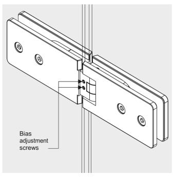
Adjust the bias on the hinges using the 2 small grub screws on the inside and outside of the hinge. For an outward opening door, the two grub screws on the outside of each hinge should be undone until their heads are flush with the hinge. The grub screws on the inside of the hinge can then be tightened, pulling the door in to the seal.
