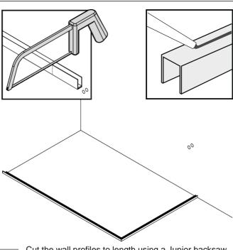
Cut the wall profiles to length using a Junior hacksaw and then file the cut ends smooth.
