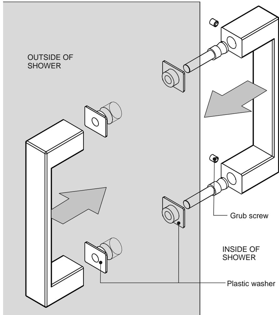
**1** If you have chosen a back-to-back handle, fit this to the door as shown, ensuring the black plastic washers are located in the holes on both sides of the glass.
