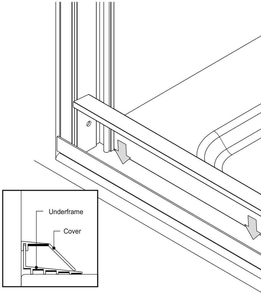
**9** Fit the Door side Underframe Cover to the Underframe. This part is intended to be removable to facilitate cleaning.
