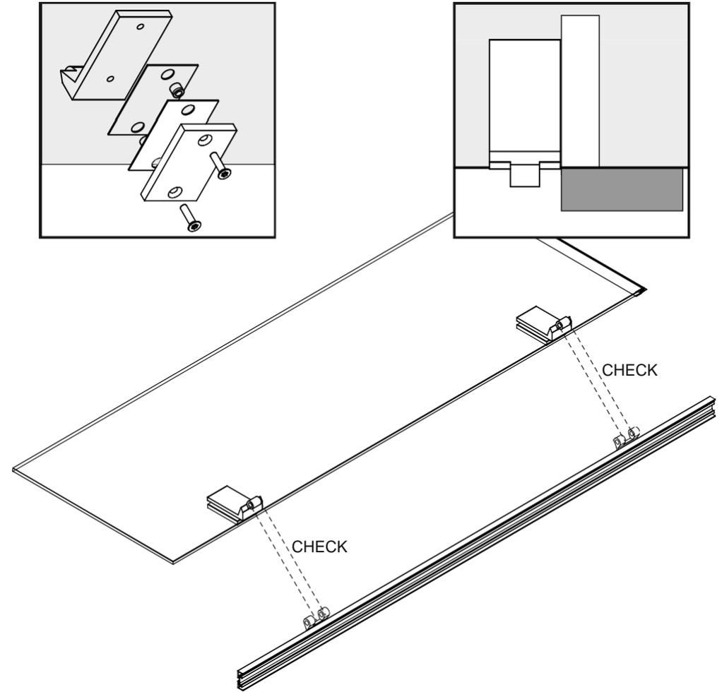
**4** Lay the glass Door horizontally on cushioned trestles or similar and assemble the hinges to the glass Door as shown. Ensure that the clear plastic sleeves are fitted inside the holes in the glass and that gaskets are placed either side of the glass.
