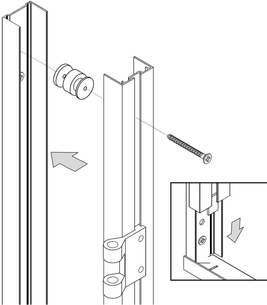
**7** Assemble the inner wall frames to the outer profiles using the longer screws provided in the remaining holes. Note that inner frames have small metal tags protruding at the bottom which are to locate in pierced slots at each end of the Underframe.
