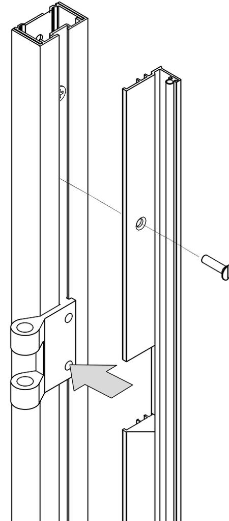
**8** Once you are satisfied that the faces of the inner wall frames are at 90 degrees to the shower base, fully tighten the wall screws and replace the cover plates as shown on both the hinge side and the handle side of the door.
