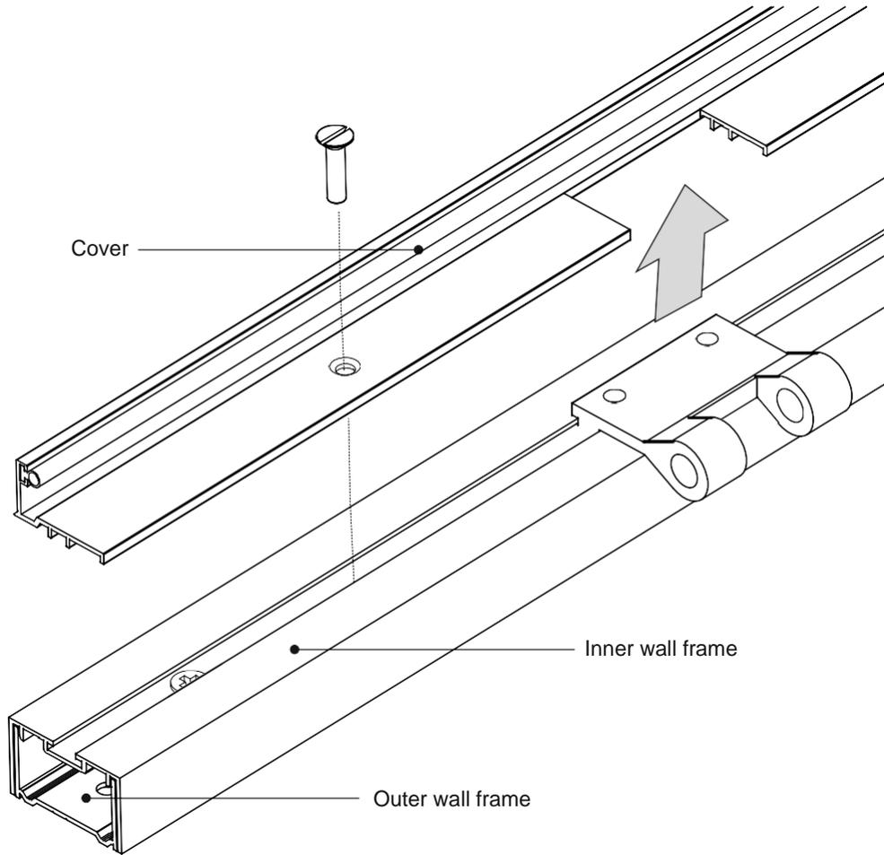
**3** Unscrew and separate the covers from the Wall Frame assemblies as shown .
