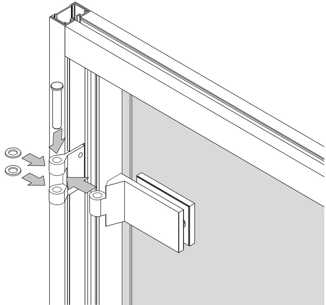
**10** Offer up the assembled Door. Place the plastic washers in between the moving parts of the hinge as shown and drop the retaining pins into place from above.
