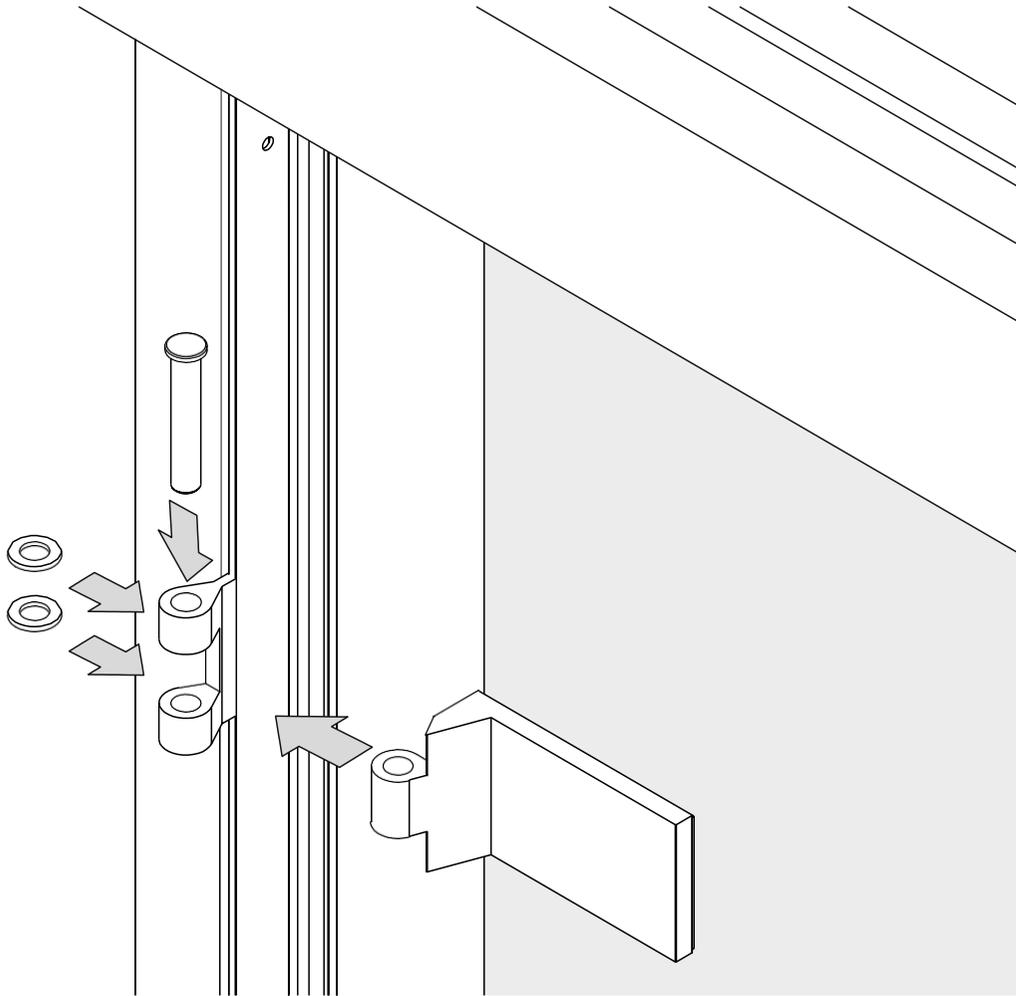
**1** Offer up the assembled Door. Place the plastic washers in between the moving parts of the hinge as shown and drop the retaining pins into place from above.
