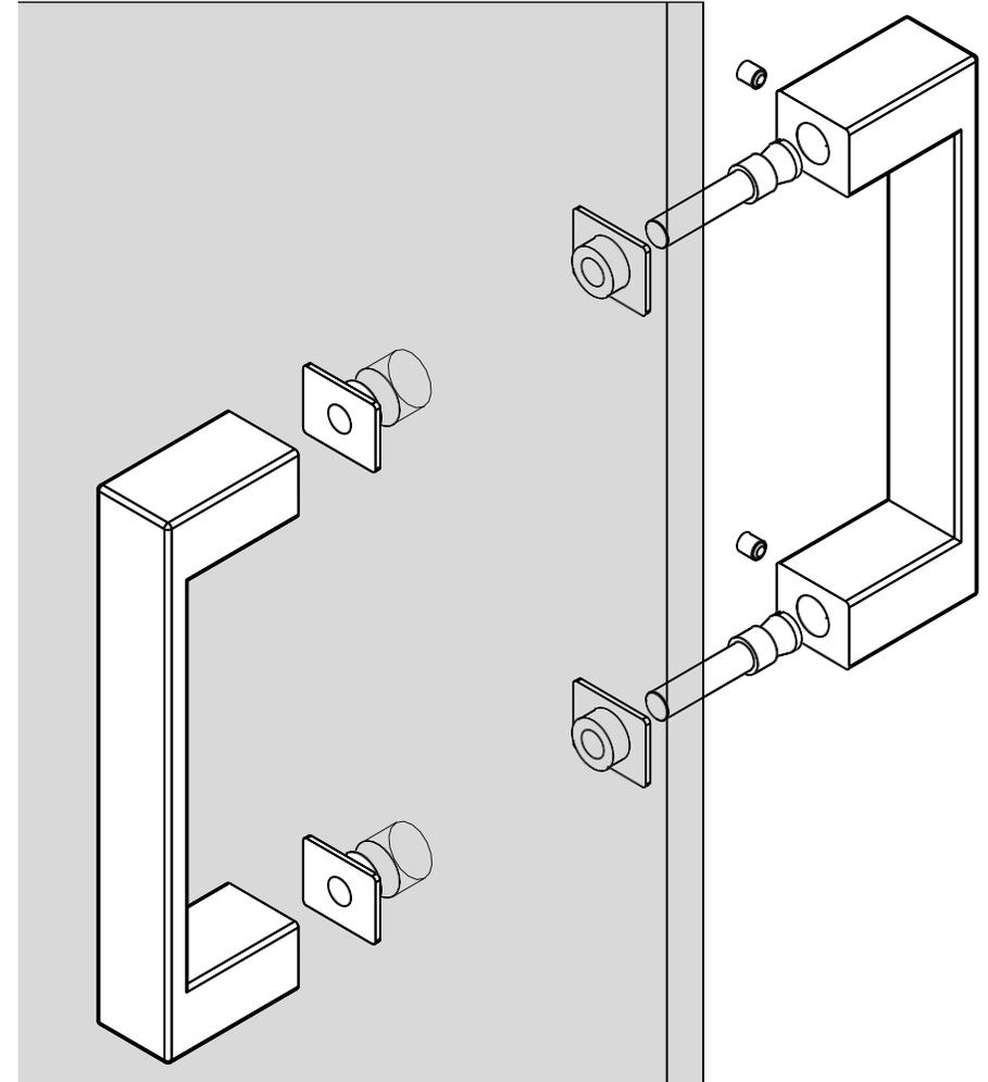
**12** If you have chosen a back-to-back handle, fit this to the door as shown, ensuring the black plastic washers are located in the holes on both sides of the glass.
