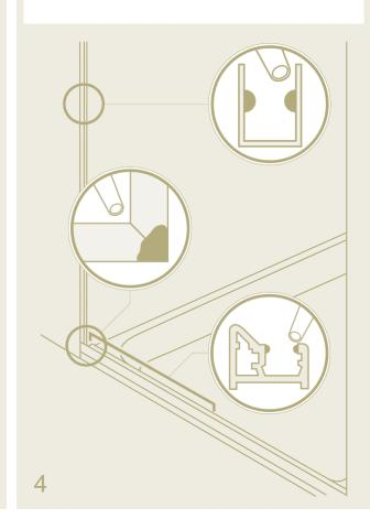
The underframe may be too long; measure the width of the opening where the shower screen is to be fitted.
