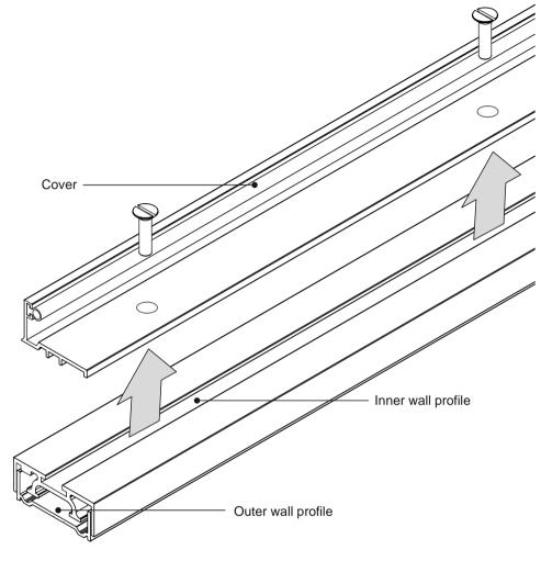
$\hfill \hfill \hfill$  Unscrew and separate the covers from the wall profile assemblies as shown .
