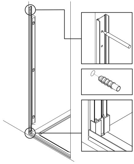
Place the outer wall profiles in position. Use the template provided to position the bottom of each outer profile and ensure that there is enough space between it and the Underframe for the inner wall profiles to be fitted later. Use a spirit level to ensure that the profiles are plumb vertical.
