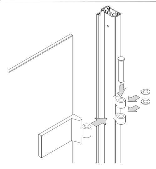
Offer up the assembled Door. Place the plastic washers in between the moving parts of the hinge as shown and drop the retaining pins into place from above.
