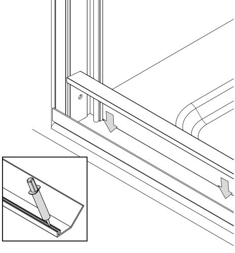
Once you are satisfied that the faces of the inner wall profiles are at 90 degrees to the shower base, fully tighten the wall screws and replace the cover plates as shown on both the hinge side and the handle side of the door.
