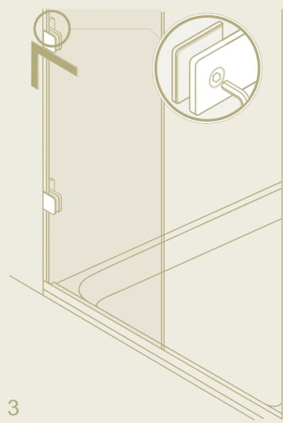
Apply continuous beads of silicone along the inside of the vertical channel and underframe channel where the glass panel will sit and into the corner joint as shown.
